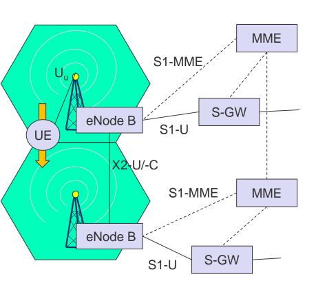
Seamless or lossless handovers possible as well as multiple target eNodeBs
