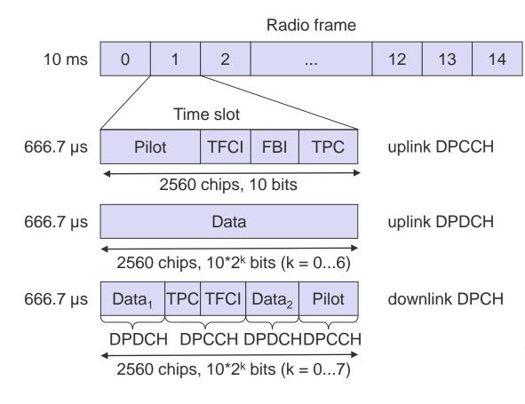
Slot structure NOT for user separation but synchronization for periodic functions!
