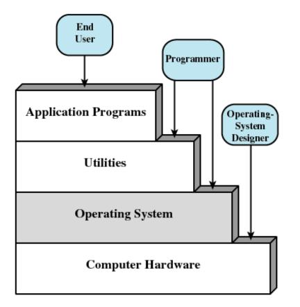
Figure 2.1 Layers and Views of a Computer System
